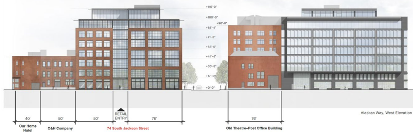
Figure xxx. An example of height analysis from a viewpoint looking into the district.
